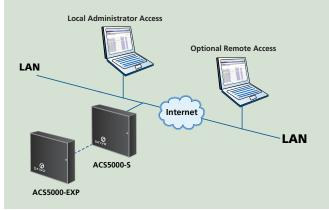
The ACS OnSite control panel can accommodate up to 30 readers. Local Administrator Access is via a Web browser over the Local Area Network (LAN). Remote Access can be set up with the appropriate network configuration, so that the system can be administered from any Web browser with Internet access.
