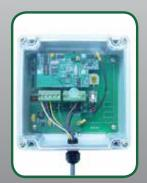
Super Long Range Active (10 to 2000 ft.) for Gate Controls, Personnel/Asset Tracking, Theft Prevention. Wiegand Output, TCP/IP, USB or Serial.
